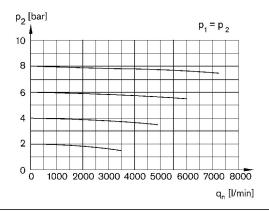
p1 = Working pressure p2 = Secondary pressure qn = Nominal flow
