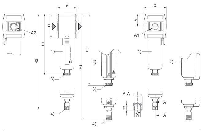
A1 = input A2 = output A7 = condensate drain 1) Plastic reservoir and protective guard with window
