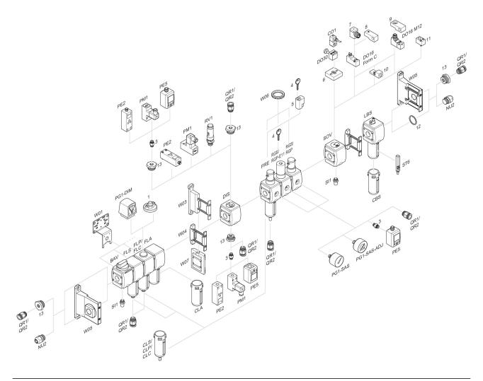
1 = contamination display 3 = Double nipple 4 = Key for E11 locking 5 = mortise lock 6 = Transition plate DO30 7 = Adapter, Series CON-VP 8 = Mounting aid DO16, form C 9 = Mounting aid DO16, M12 10 = Adapter for external pilot air 11 = Adapter pneumatic operation 12 = Sealing ring 13 = Reducing nipple
