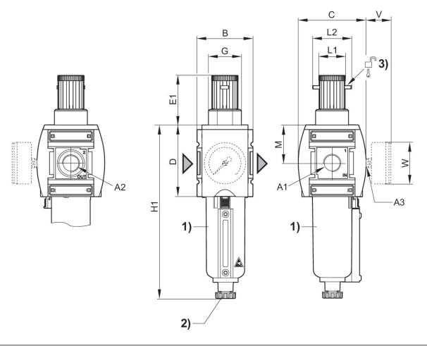
A1 = input A2 = output A3 = pressure gauge connection
