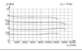
p1 = Working pressure p2 = Secondary pressure
