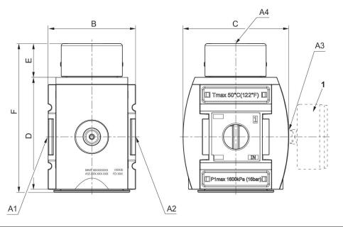
A1 = input A2 = output A3 = pressure gauge connection
