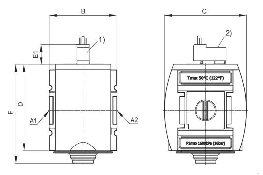
A1 = input A2 = output 1) Connection for valve plug connector according to ISO 15217 (form C) 2) Manual override
