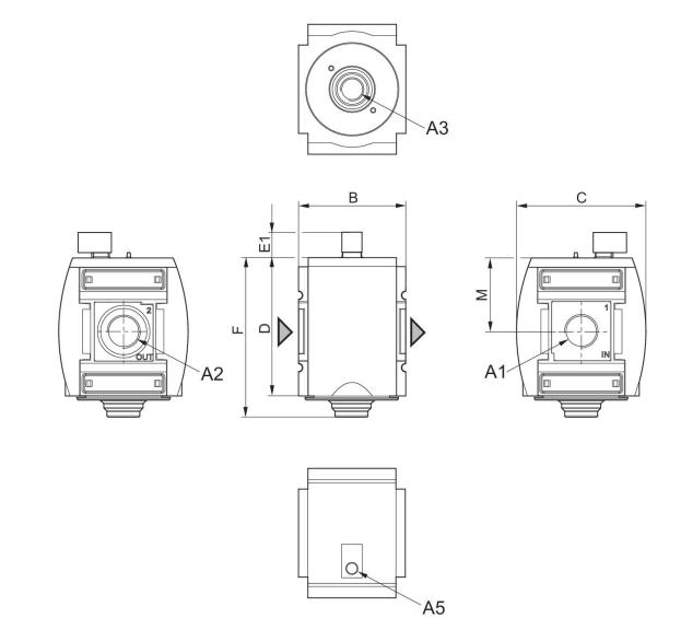
A1 = input A2 = output A3 = ventilation port A5 = control pressure connection
