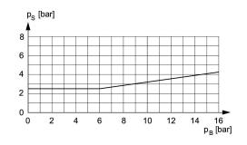
minimum pilot pressure depending on working pressure PS = control pressure  $P_B$  = Working pressure
