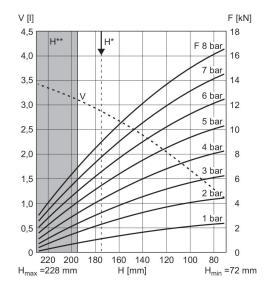
V = volume H = height H\* = recommended operating height for vibration isolation H\*\* = use permitted only upon approval by AVENTICS 1 kN = 1000 N
