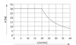
Max. permissible radial bearing load F during switching operation Ø 32 mm
