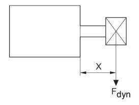
F dyn. = dynamic lateral force X = distance between force application point and cylinder cover S = stroke
