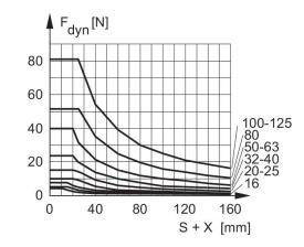
F dyn. = dynamic lateral force X = distance between force application point and cylinder cover S = stroke
