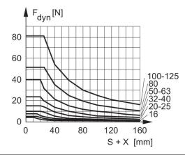
F dyn. = dynamic lateral force X = distance between force application point and cylinder cover S = stroke
