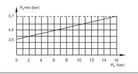
P<sub>B</sub> = Working pressure PS = control pressure
