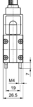
1) not assigned 2) magnet 12 3) 0 V 4) magnet 14 5) metal round plug M12x1 6) positioning pin 7) yellow valve switching state LED 9) manual override
