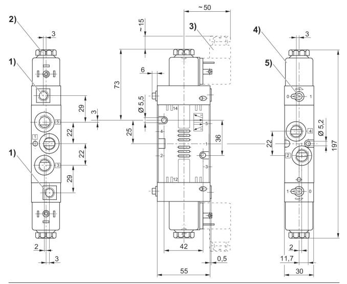
1) Only with separate pilot control G 1/8 2) After removal of cap M5 internal thread 3) Valve plug connector 4) Coil can be plugged at 45° intervals 5) Manual override
