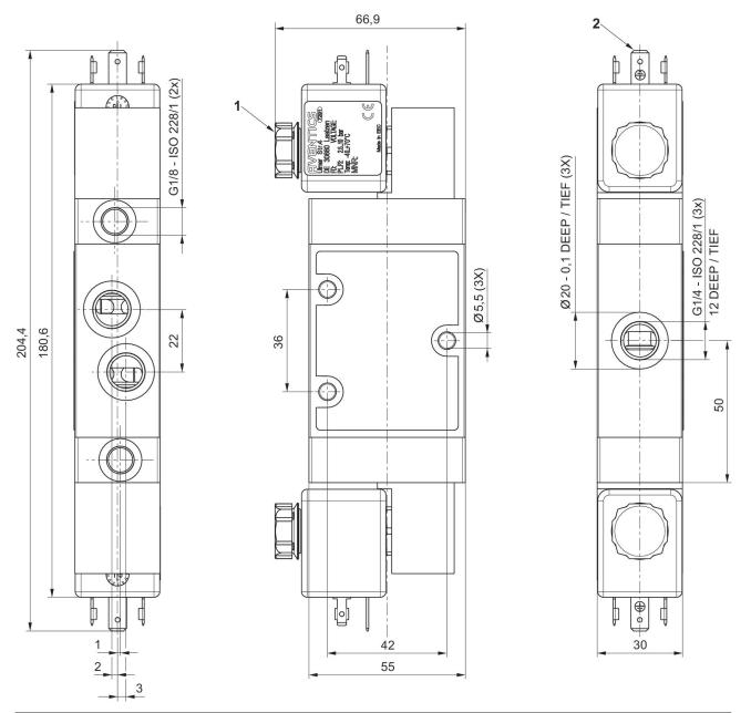
1) Silencer 2) Valve plug connector form A, EN 175301-803
