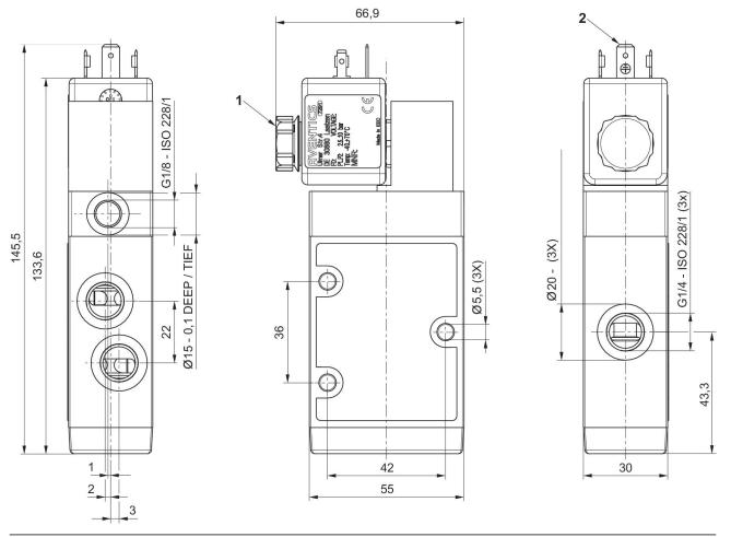
1) Silencer 2) Valve plug connector form A, EN 175301-803
