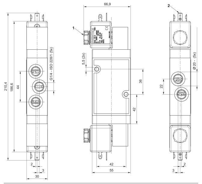
1) Silencer 2) Valve plug connector form A, EN 175301-803
