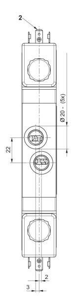
1) Silencer 2) Valve plug connector form A, EN 175301-803
