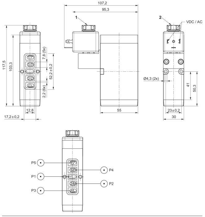
1) Silencer 2) Valve plug connector form A, EN 175301-803
