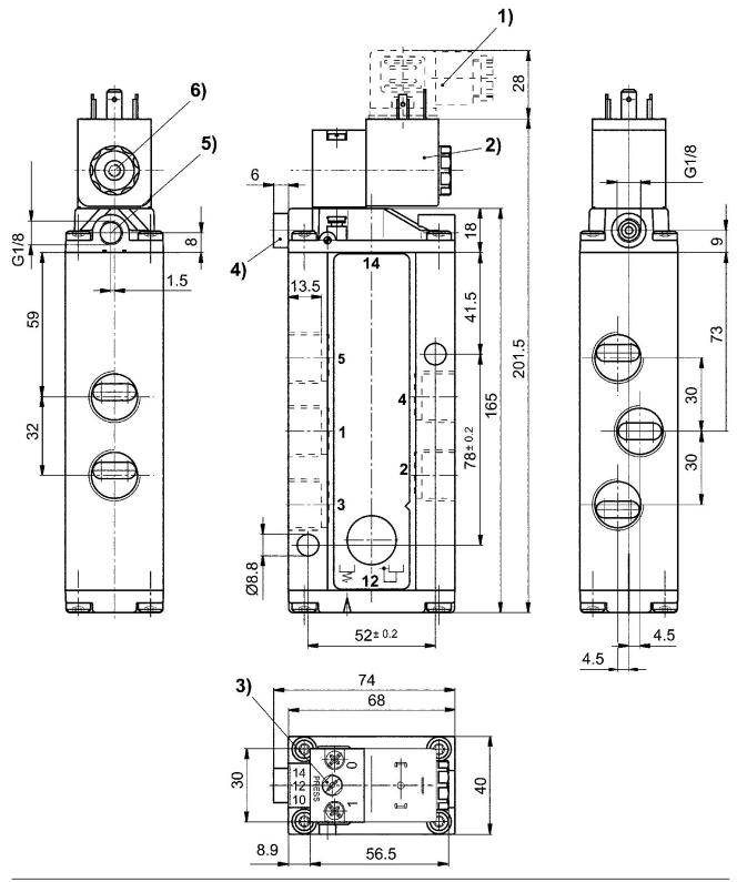
Valve plug connector 2) Coil can be rotated at 90° intervals 3) Manual override
