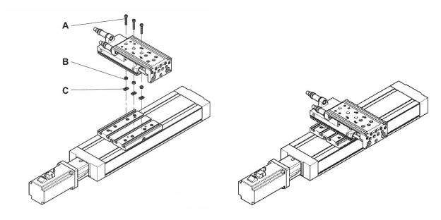
Scope of delivery: A) screws B) centering sleeves C) sliding blocks
