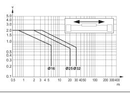
$v_t$  = Piston velocity [m/s] m = Cushionable mass [kg]
