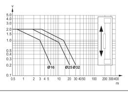
v<sub>t</sub> = Piston velocity [m/s] m = Cushionable mass [kg]
