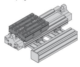
fastening of automation system Easy2Combine to CKP using center rings and T-groove nuts (example: mini slide MSC)
