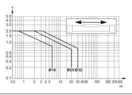
$v_t$  = Piston velocity [m/s] m = Cushionable mass [kg]
