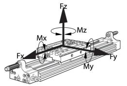
With simultaneously moments on the cylinder this equation must be used in addition to the maximum moments check. In the cushioning phase of the movement additional forces occur and must be considered. Please use our calculation tool for rodless cylinders on the http://www.aventics.com.
