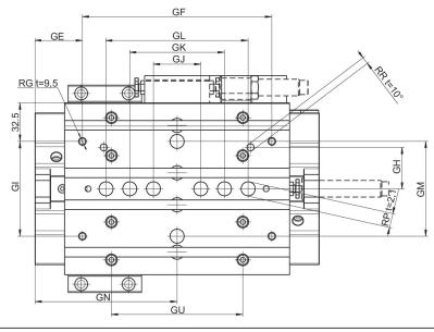
− t = depth \* CKP 16: 2x Lube ports on each runner block, CKP 25 / 30: Lube nipple of funnel type with thread connection M3
