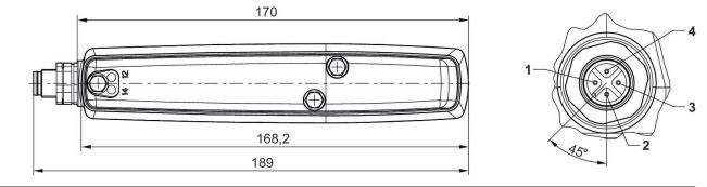
Electrical connection: 1) Not connected 2) Solenoid 12 3) 0 V 4) Solenoid 14
