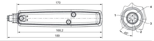
Electrical connection: 1) Not connected 2) Solenoid 12 3) 0 V 4) Solenoid 14
