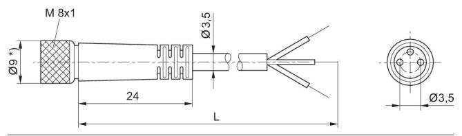
L = length \*) With 15 m cable length Ø12
