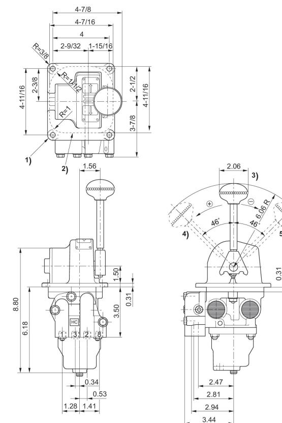
1) Mounting hole Ø11/32 2) panel mounting hole
