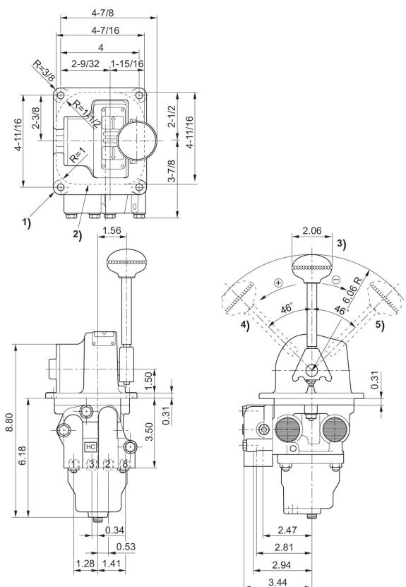
1) Mounting hole Ø11/32 2) panel mounting hole
