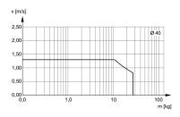
v = Piston velocity [m/s] m = Cushionable mass [kg]
