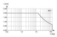
v = Piston velocity [m/s] m = Cushionable mass [kg]
