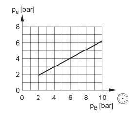
Pe = external control pressure, min.
