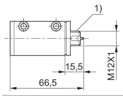
1) not intended as mounting thread Mounting via 2 through-holes in housing
