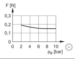
${\sf F}$  = actuating force at the rear end of the spring-loaded rod  ${\sf P}_{\sf B}$  = Working pressure
