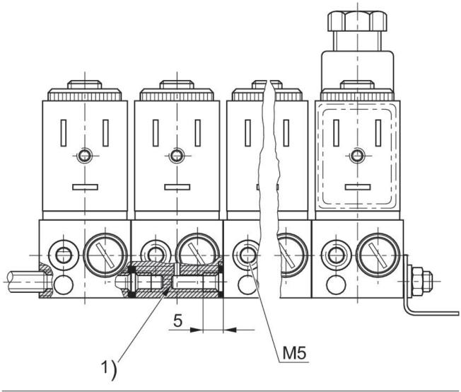
Before assembly, the blanking tab must be broken through with a punch (Ø4 mm).
