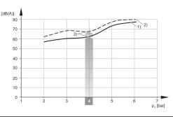
1) Ø nozzle [[1.0] mm] 2) Ø nozzle [[1.5] mm]
