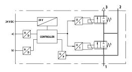
a) Nominal input value b) Actual output value The E/P pressure control valve modulates the pressure corresponding to an analog electrical nominal input value.
