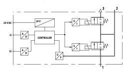
a) Nominal input value b) Actual output value The E/P pressure control valve modulates the pressure corresponding to an analog electrical nominal input value.
