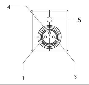
Pin assignment (1) Pin not assigned (3) 0 V (4) 24 V (5) LED Note: Bipolar protective circuit to prevent overvoltage
