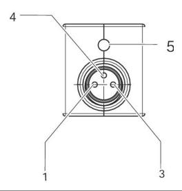
Pin assignment (1) Pin not assigned (3) 0 V (4) 24 V (5) LED Note: Bipolar protective circuit to prevent overvoltage
