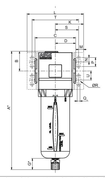
\*Variable dimension based on the type of drain specified, if an automatic drain is specified, add another [[5] mm] to the "G" dimension, which also adds 5 mm to the "A" dimension.
