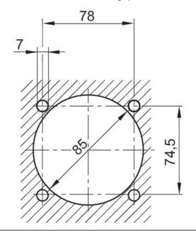
Mounting plate max. 10 mm thick
