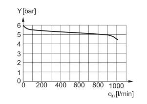
input pressure: 8 bar, supply pressure: 6 bar y: pressure in line "A" [bar]
