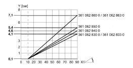
$\begin{array}{l} {\sf x} = {\sf lever path} \\ {\sf The characteristic curve can be moved parallel to the illustrated} \\ {\sf characteristic curve (in the y direction) using the screw cap.} \end{array}$
