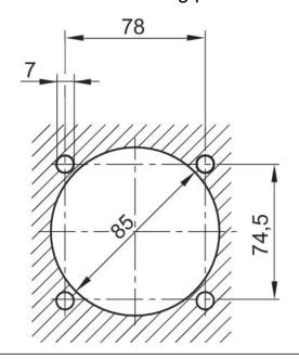
Mounting plate max. 10 mm thick
