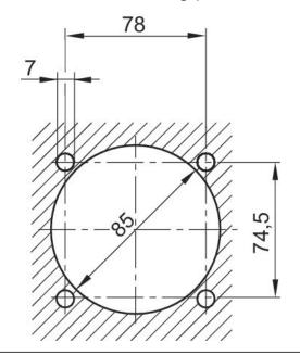
Mounting plate max. 10 mm thick
