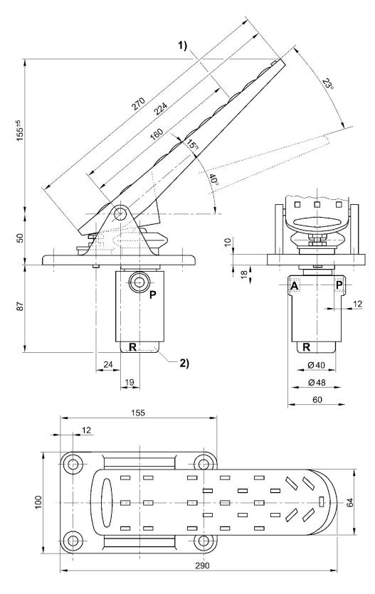
1) actuating force on the pedal 2) Screw cap
