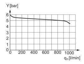
input pressure: 8 bar, supply pressure: 6 bar y: pressure in line "A" [bar]
