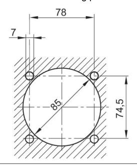
Mounting plate max. 10 mm thick
